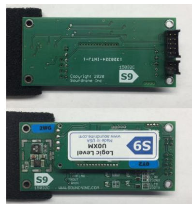
Figure 6: OEM Ultimodem; SBE IMM Compatible footprint with power supply
